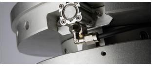
The bottom ring is equipped with pneumatic actuators which are directly driven by the control system. When the mast is extended, they automatically lock the section; when the mast has to be retracted, the section can't be unlocked if the air supply is missing or if the inner pressure has not reached the safety value. As soon as both conditions are met, the retraction sequence in both automatic and manual modes can be safely started.
